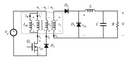
Fig. 6.23 Forward converter, with transformer equivalent circuit model.
