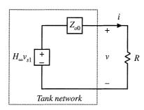
Fig. 19.31 Thevenin-equivalent circuit that models the output port of the tank network.
