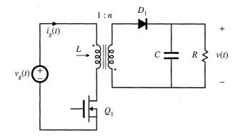
Fig. 7.18 Flyback converter example.
