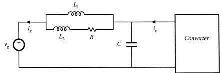
Fig. 8.28 Input EMI filter example.
