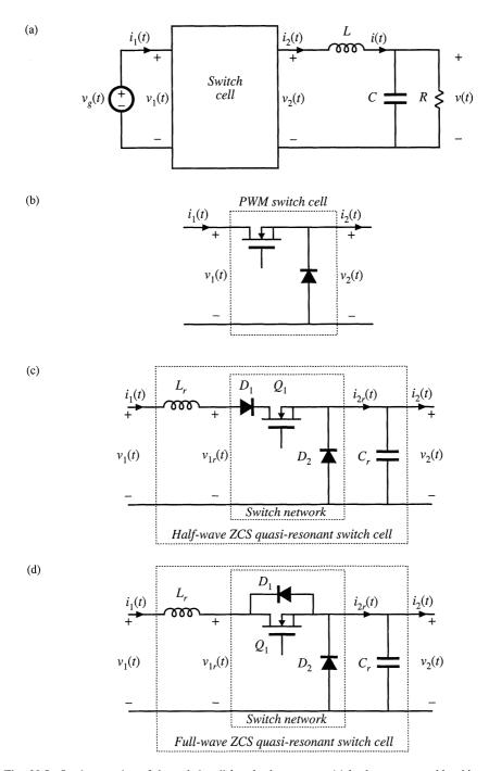
**Fig. 20.8** Implementation of the switch cell in a buck converter: (a) buck converter, with arbitrary switch cell; (b) PWM switch cell; (c) half-wave ZCS quasi-resonant switch cell; (d) full-wave ZCS quasi-resonant switch cell.
