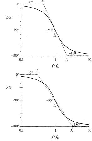
**Fig. 8.23** A simpler choice for the midfrequency phase asymptote, which better approximates the curve over the entire frequency range and is consistent with the asymptote used for real poles.
