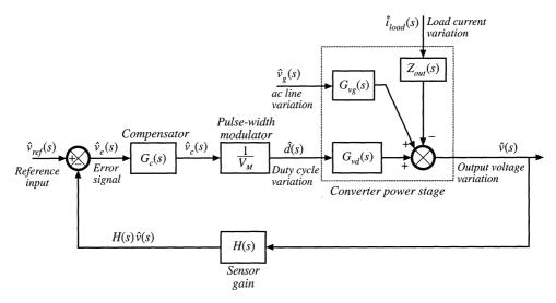
Fig. 9.4 Voltage regulator system small-signal model: (a) with converter equivalent circuit; (b) complete block diagram.
