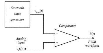
Fig. 7.63 A simple pulse-width modulator circuit.
