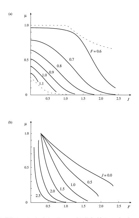
**Fig. 20.27** Conversion ratio  $\mu$  for the multi-resonant switch with  $C_d = 3C_s$ : (a) conversion ratio  $\mu$  vs. normalized current *J* (solid lines: conversion ratio; dashed lines: boundaries of zero-voltage switching), (b) conversion ratio  $\mu$  vs. normalized switching frequency *F*.
