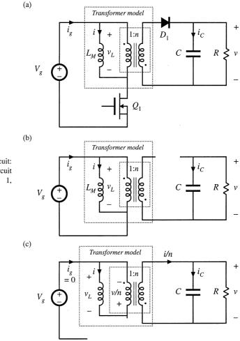
**Fig. 6.31** Flyback converter circuit: (a) with transformer equivalent circuit model, (b) during subinterval 1, (c) during subinterval 2.
