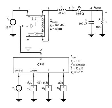
Fig. B.25 CPM buck converter example.
