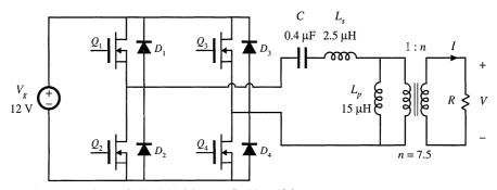
Fig. 19.56 Transformer-isolated LLC inverter, Problem 19.9.
