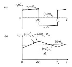
Fig. 7.20 Inductor waveforms for the flyback example: (a) inductor voltage, (b) inductor current.
