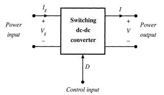
Fig. 3.1 Switching converter terminal quantities.
