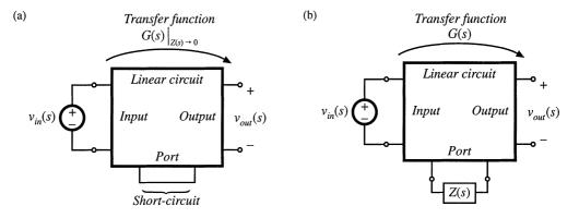
Fig. C.2 The dual form of the Extra Element Theorem, in which the extra element replaces a short circuit: (a) original conditions, (b) addition of element having impedance Z(s).
