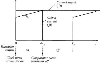
to the input of a compensation network, and the output of the compensator drives the control signal  $i_c(t)R_f$ . To design such a feedback system, we need to model how variations in the control signal  $i_c(t)$  and in the line input voltage  $v_o(t)$  affect the output voltage v(t).
