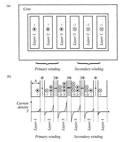
Fig. 13.25 A simple transformer example illustrating the proximity effect: (a) core and winding geometry, (b) distribution of currents on surfaces of conductors.
