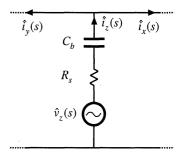
$\hat{v}_z$  and output resistance  $R_s$ . A series capacitor,  $C_b$ , is inserted to avoid disrupting the dc bias at the injection point.
