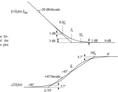
Fig. 8.15 Inversion of the frequency axis: summary of the magnitude and phase Bode plot for the inverted real zero.
