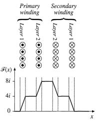
It should be noted that the shape of the  $\mathcal{F}(x)$  curve in the vicinity of the winding conductors depends on the distribution of the current within the conductors. Since this distribution is not yet known, the  $\mathcal{F}(x)$  curve of Fig. 13.28 is arbitrarily drawn as straight line segments.
