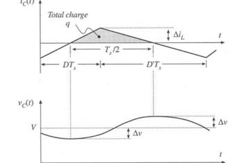
Fig. 2.26 Output capacitor voltage and current waveforms, for the buck converter in Fig. 2.25.
