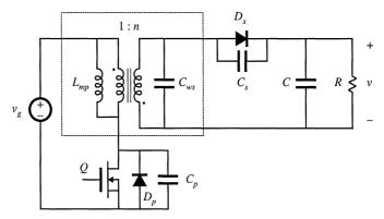
Fig. 20.44 High-voltage dc–dc converter containing a resonant switch network, Problem 20.2.
