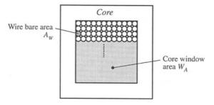
Fig. 14.5 The winding must fit in the core window area.
