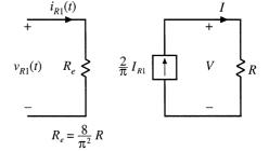
The rectified tank output current,  $|i_R(t)|$ , is filtered by capacitor  $C_F$ . Since no dc current can pass through  $C_F$ , the dc component of  $|i_R(t)|$  must be equal to the steady-state load current *I*. By equating dc components we obtain:
