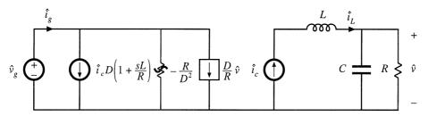
Fig. 12.21 Simplification of the CPM buck converter model of Fig. 12.19, with dependent source expressed in terms of the output voltage variations.
