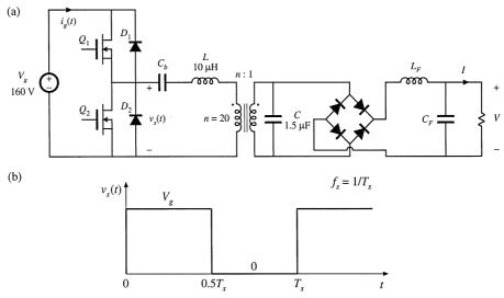
Fig. 19.53 Half-bridge parallel resonant converter of Problem 19.1: (a) schematic, (b) switch voltage waveform.
