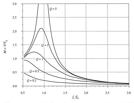
Fig. 19.52 Exact control characteristics of the parallel resonant converter, with a resistive load. Both CCM and DCM operation is included, for  $0.5 \le F \le 3$ .
