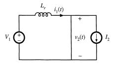
Fig. 20.11 Circuit of the switch network during subinterval 1.
