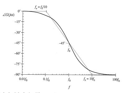
Fig. 8.10 A simpler choice for the midfrequency phase asymptote, which better approximates the curve over the entire frequency range.
