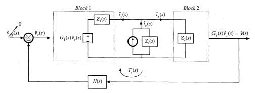
Fig. 9.38 Measurement of loop gain by current injection.
