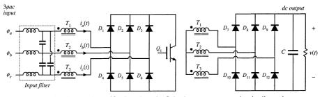
Fig. 18.45 Isolated 3øac–dc rectifier based on the flyback converter operating in discontinuous conduction mode: Problem 18.9.
