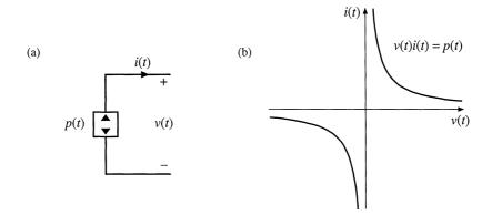
Fig. 11.5 The dependent power source: (a) schematic symbol, (b) *i*-*v* characteristic.
