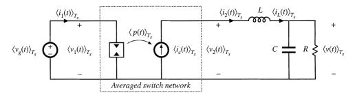
Fig. 12.17 Averaged model of CPM buck converter.
