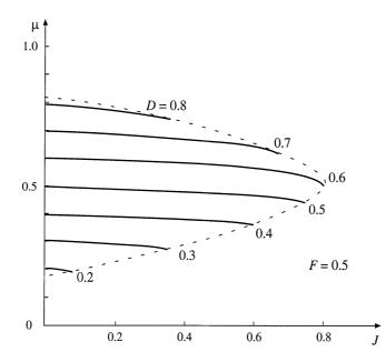
Fig. 20.35 Conversion ratio  $\mu$ , as a function of duty cycle *D* and normalized load current *J*, for the two-switch QSW-ZVS switch illustrated in Fig. 20.33. Curves are plotted for constant-frequency control with F = 0.5. The dashed line is the zero-voltage switching boundary.
