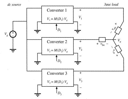
Fig. 6.12 Generation of dc–3¢ac inverter by differential connection of 3¢ load.
