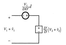
The term  $(V_1/DD')\hat{d}(t)$  is driven by the control input  $\hat{d}$ , and hence can be represented by an independent voltage source as in Fig. 7.40. The term  $(D'/D)(V_2 + \hat{v}_2(t))$  is equal to the constant value (D'/D) multiplied by the port 2 independent voltage  $(V_2 + \hat{v}_2(t))$ . This term is represented by a dependent voltage source in Fig. 7.40. This dependent source will become the primary winding of an ideal transformer.
