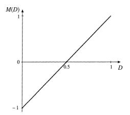
Fig. 6.12 Conversion ratio of the H-bridge inverter circuit.
