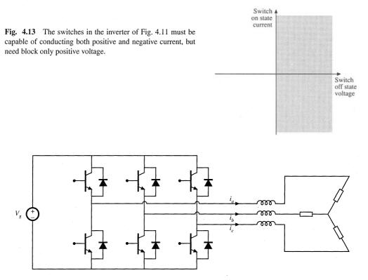
Fig. 4.14 The dc-3øac voltage-source inverter requires two-quadrant switches.
