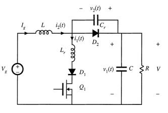
Fig. 20.17 Boost converter containing a half-wave ZCS quasi-resonant switch.
