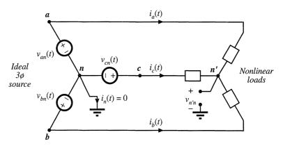
Fig. 16.10 Current flow in a three-phase three-wire wye-connected network.
