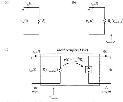
**Fig. 18.1** Development of the ideal rectifier equivalent circuit model: (a) input port resistor emulation; (b) the value of the emulated resistance, and hence the power throughput, is controllable; (c) output port power source characteristic, and complete model.
