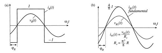
Fig. 19.20 Rectifier network input terminal waveforms, for the parallel resonant converter: (a) actual waveforms  $v_R(t)$  and  $i_R(t)$ , (b) fundamental components  $v_{R1}(t)$  and  $i_{R1}(t)$ .
