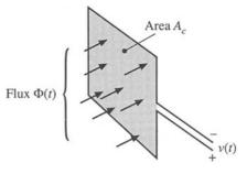
Fig. 13.2 The voltage v(t) induced in a loop of wire is related by Faraday's law to the derivative of the total flux  $\Phi(t)$  passing through the interior of the loop.
