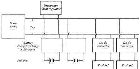
Fig. 1.15 Power system of an earth-orbiting spacecraft.
