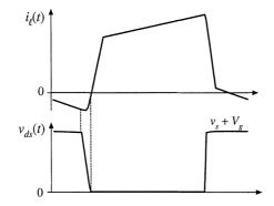
Fig. 20.40 Waveforms of the active-clamp snubber circuit of Fig. 20.39(a).
