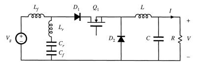
**Fig. 20.29** Incorporation of a ZCS quasi-square-wave resonant switch into a buck converter containing an *L*–*C* input filter.
