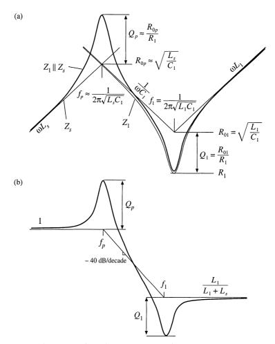
Fig. 17.21 Construction of approximate frequency response using the algebra-on-the-graph method: (a) impedance asymptotes, (b) transfer function asymptotes || H ||.
