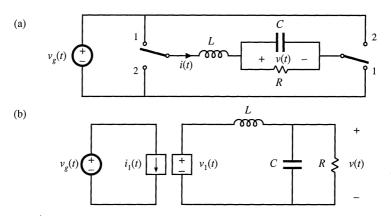
Fig. 7.69 Bridge inverter, Problem 7.11: (a) circuit, (b) large-signal averaged model.
