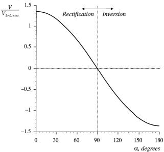
Fig. 17.13 Variation of the dc output voltage V with delay angle  $\alpha$ , for the phase-controlled circuit of Fig. 17.11.
