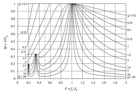
Fig. 19.45 Complete control plane characteristics of the series resonant converter, for the range  $0.2 \le F \le 2$ .
