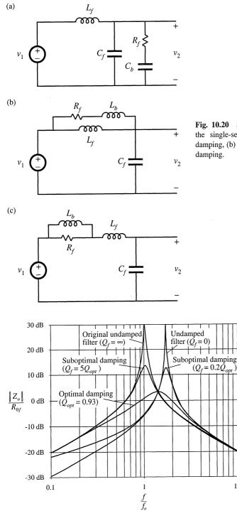
**Fig. 10.20** Several practical approaches to damping the single-section input filter: (a)  $R_f - C_b$  parallel damping, (b)  $R_f - L_b$  parallel damping, (c)  $R_f - L_b$  series damping.
