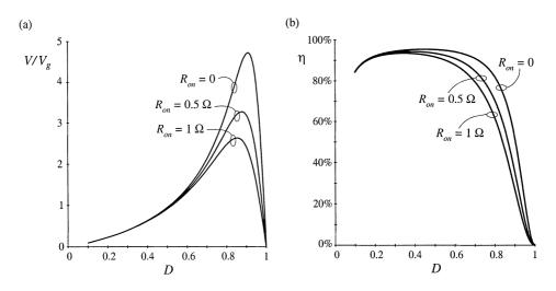
Fig. B.5 SEPIC simulation example: (a) dc conversion ratio and (b) efficiency.
