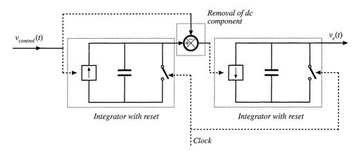
Fig. 18.23 Generation of parabolic carrier waveform by double integration.
