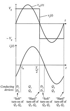
transistor on. With a minor circuit modification, the transistor turn-off transitions can also be caused to occur at zero voltage. This process can lead to significant reductions in the switching losses of converters based on MOSFETs and diodes.
