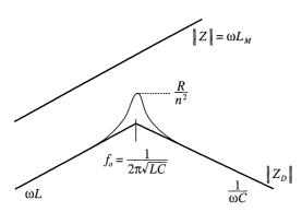
**Fig. C.16** To avoid significantly changing the transfer function G(s), the transformer should be designed such that  $||Z|| \gg ||Z_D||$ .
