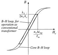
In the transformer application, core loss and proximity losses are usually significant. Typically the maximum flux density is limited by core loss rather than by saturation. A high-frequency material having low core loss is employed. Both core and copper losses must be accounted for in the design of the transformer. The design must also incorporate multiple windings. Transformer design with flux density optimized for minimum total loss is described in Chapter 15.
