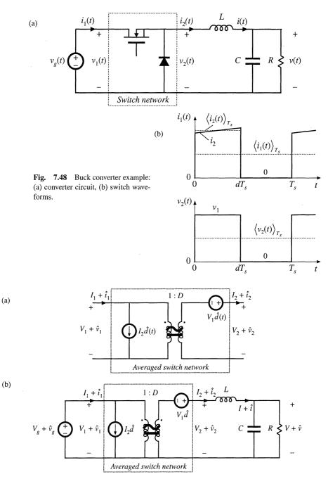
Fig. 7.49 Averaged switch modeling, buck converter example: (a) dc and small-signal ac averaged switch model; (b) Averaged circuit model of the buck converter obtained by replacement of the switch network by the averaged switch model.
