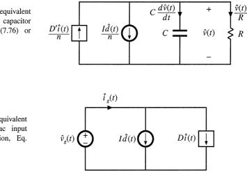
small-signal transfer functions is modeled by an effective resistance of value  $DR_{on}$ .
