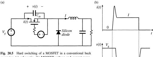
Fig. 20.5 Hard switching of a MOSFET in a conventional buck converter: (a) schematic, (b) MOSFET voltage and current wave-forms.
