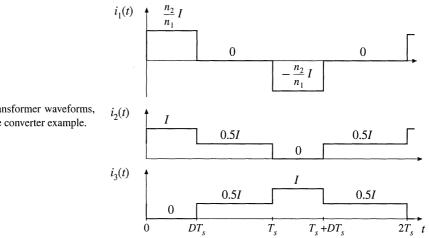
Fig. 14.10 Transformer waveforms, PWM full-bridge converter example.
