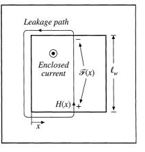
Fig. 13.28 MMF diagram for the transformer winding example of Figs. 13.26 and 13.27.
