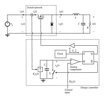
Fig. 12.37 Buck converter with charge controller, Problem 12.11.
