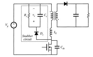
Fig. 20.6 Insertion of a dissipative voltage-clamped snubber circuit into a flyback converter. The MOSFET voltage is clamped to a peak value of  $(V_g + v_s)$ .
