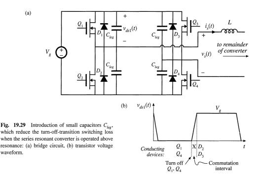
Ringing is conspicuously absent from the waveforms of converters in which all semiconductor devices switch at zero voltage; these converters inherently do not generate this type of EMI.
