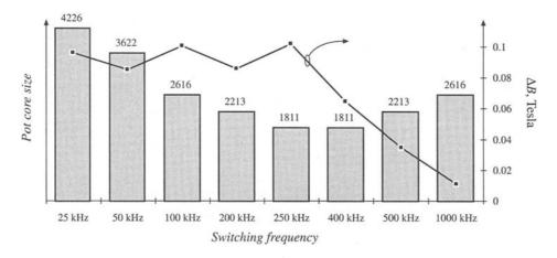
Fig. 15.7 Variation of transformer size (bar chart) with switching frequency, Ćuk converter example. Optimum peak ac flux density (data points) is also plotted.
