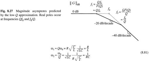
by the low-Q approximation. Real poles occur at frequencies  $Qf_0$  and  $f_0/Q$ .
