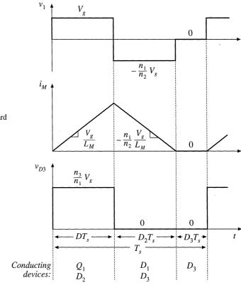
Fig. 6.24 Waveforms of the forward converter.
