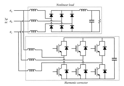
Fig. 18.43 A harmonic corrector, based on the 3øac-dc CCM boost converter of Fig. 18.39.
