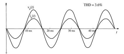
Fig. 17.6 Typical ac line current and voltage waveforms, near the boundary between continuous and discontinuous modes and with small dc filter capacitor.  $f_0/f_L = 10$ , Q = 1.
