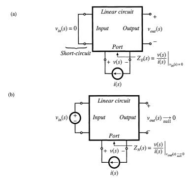
Fig. C.3 Determination of the quantities  $Z_N(s)$  and  $Z_D(s)$ : (a)  $Z_D(s)$  is the Thevenin-equivalent impedance at the port, and is measured with the input  $v_{in}(s)$  set to zero; (b)  $Z_N(s)$  is the impedance seen at the port under the condition that the output is nulled.
