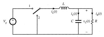
Fig. 2.25 The buck converter contains a two-pole output filter.
