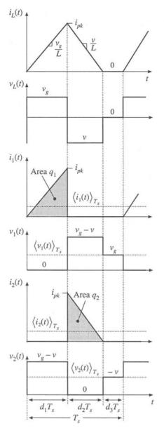
Fig. 11.3 Inductor and switch network voltage and current waveforms.
