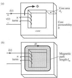
Fig. 13.8 Inductor example: (a) inductor geometry, (b) application of Ampere's law.
