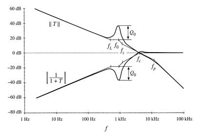
Fig. 9.31 Construction of ||T|| and ||1/(1 + T)|| with the *PID*-compensator of Fig. 9.30.
