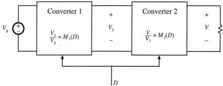
Fig. 6.3 Cascade connection of converters.
