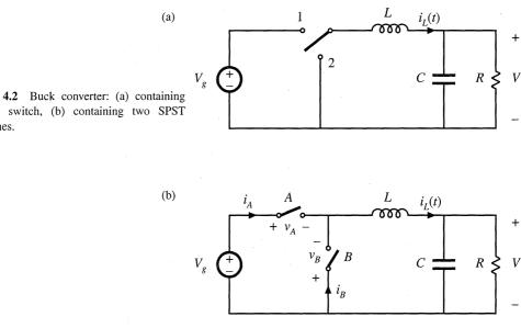
SPDT switch, (b) containing two SPST switches.
