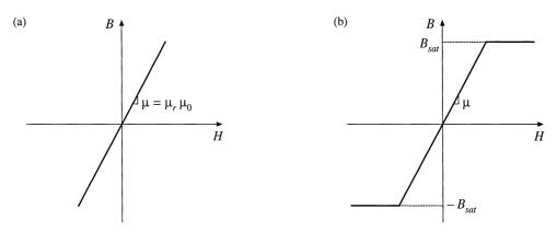
Fig. 13.6 Approximation of the B-H characteristics of a magnetic core material: (a) by neglecting both hysteresis and saturation, (b) by neglecting hysteresis.
