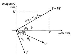
Fig. 16.8 Power phasor diagram, for a sinusoidal system, illustrating the voltage, current, and complex power phasors.
