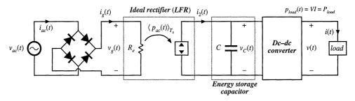
**Fig. 18.25** Elements of a single-phase-ac to dc power supply, in which the ac line current and dc load voltage are independently regulated with high bandwidth. An internal independent energy storage capacitor is required.
