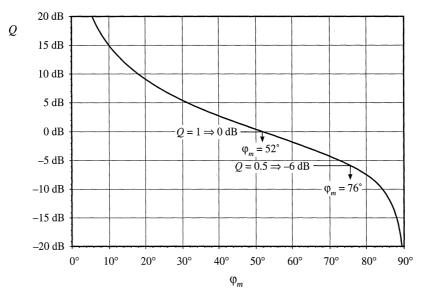
Fig. 9.13 Relationship between loop-gain phase margin  $\varphi_m$  and closed-loop peaking factor Q.
