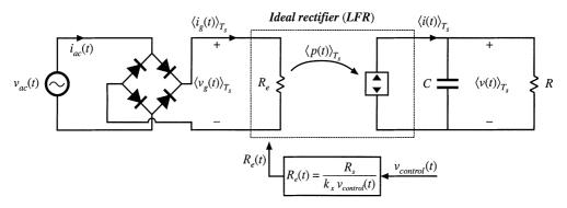
**Fig. 18.12** Model of the system of Fig. 18.5, based on the loss-free resistor model of Fig. 18.1(c), which predicts the low-frequency system waveforms. This model assumes that the feedback loop of Fig. 18.5 operates ideally.
