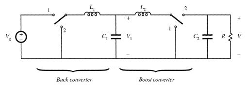
Fig. 6.4 Cascade connection of buck converter and boost converter.
