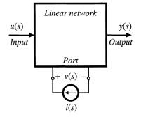
Fig. C.5 Current injection at the electrical port, by addition of independent current source i(s).
