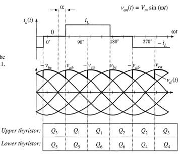
Fig. 17.12 Waveforms for the controlled rectifier of Fig. 17.11, with large dc filter inductance.
