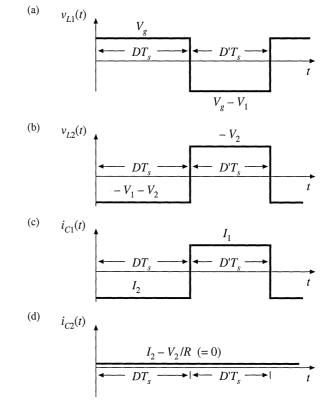
Fig. 2.22 Ćuk converter waveforms: (a) inductor voltage  $v_{L1}(t)$ , (b) inductor voltage  $v_{L2}(t)$ , (c) capacitor current  $i_{C1}(t)$ , (d) capacitor current  $i_{C2}(t)$ .
