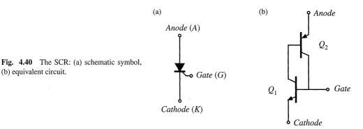
The schematic symbol of the SCR is illustrated in Fig. 4.40(a), and an equivalent circuit containing NPN and PNP BJT devices is illustrated in Fig. 4.40(b). A cross-section of the silicon chip is illustrated in Fig. 4.41. Effective transistor  $Q_1$  is composed of the *n*, *p*, and *n*<sup>-</sup> regions, while effective transistor  $Q_2$  is composed of the *p*, *n*<sup>-</sup>, and *p* regions as illustrated.
