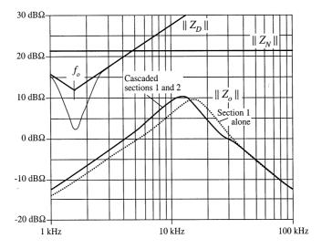
**Fig. 10.27** Comparison of the impedance design criteria  $||Z_N(j\omega)||$  and  $||Z_D(j\omega)||$ , Eq. (10.13), with the filter output impedance  $||Z_n(j\omega)||$ . Solid line:  $||Z_n(j\omega)||$  of cascaded design. Dashed line:  $||Z_n(j\omega)||$  of section 1 alone.
