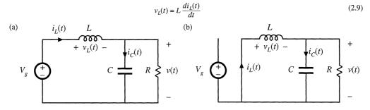
Fig. 2.8 Buck converter circuit: (a) while the switch is in position 1, (b) while the switch is in position 2.
