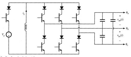
Fig. 4.18 Dc-3øac buck-boost inverter.
