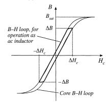
Fig. 13.44 Operational *B*–*H* loop of an ac inductor.
