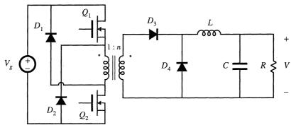
Fig. 6.27 Two-transistor forward converter.
