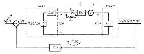
Fig. 9.40 Measurement of an unstable loop gain by voltage injection.
