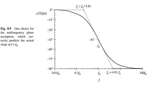
trated in Fig. 8.9, where the slope of the asymptote is chosen to be identical to the slope of the actual curve at  $f = f_0$ . It can be shown that, with this choice, the asymptote intersection frequencies  $f_a$  and  $f_b$  are given by
