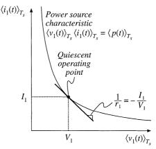
incremental resistance  $r_1$ : the slope of the power sink characteristic, evaluated at the quiescent operating point.
