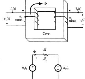
Fig. 13.13 A two-winding transformer.
