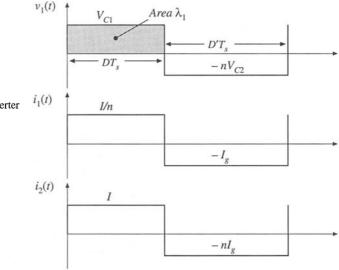
**Fig. 15.6** Waveforms, Ćuk converter  $l_1(l)$  transformer design example.
