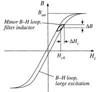
equal to the dc component *I*. Typically, the core loss can be ignored, and the design is driven by the copper loss. The maximum flux density is limited by saturation of the core. Proximity losses are negligible. Although a high-frequency ferrite material can be employed in this application, other materials having higher core losses and greater saturation flux density lead to a physically smaller device. Design of a fil-
