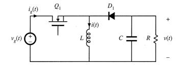
Fig. 7.31 Buck-boost converter example.
