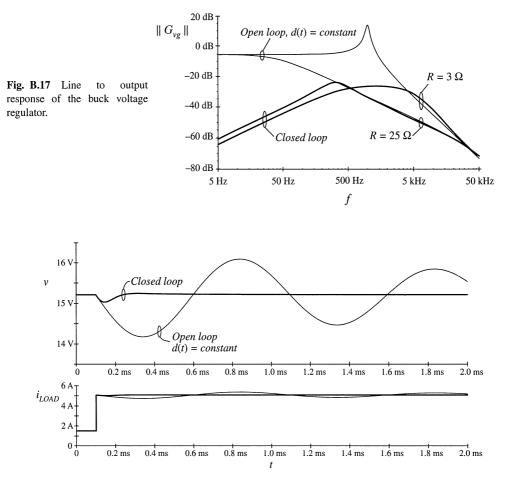
Fig. B.18 Load transient response of the buck voltage regulator example.
