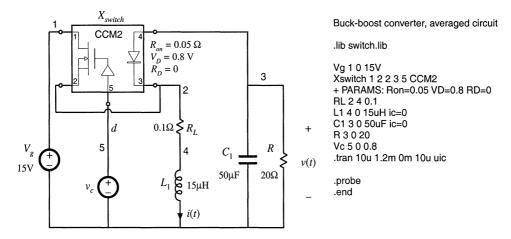
Fig. B.8 Buck-boost converter simulation example, averaged circuit model.
