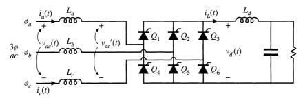
Fig. 17.16 Controlled 3ø rectifier circuit, with small ac-side inductances.
