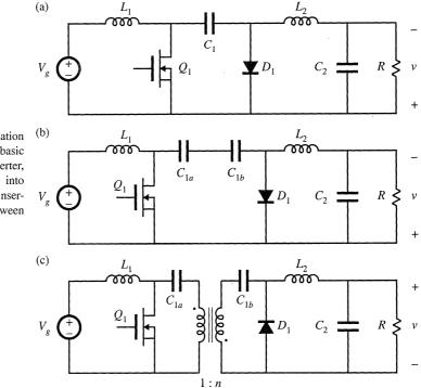
**Fig. 6.40** Obtaining isolation in the Ćuk converter: (a) basic nonisolated Ćuk converter, (b) splitting capacitor  $C_1$  into two series capacitors, (c) insertion of transformer between capacitors.
