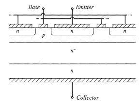
Fig. 4.30 Power BJT structure. Crosshatched regions are metallized contacts.
