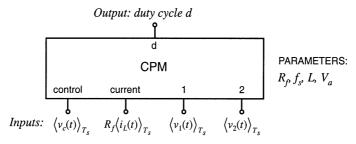
Fig. B.24 Current programmed mode (CPM) subcircuit.
