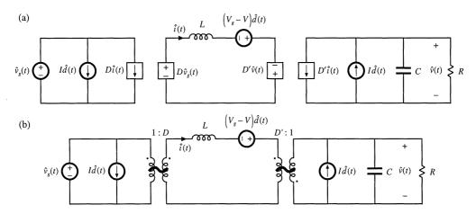
Fig. 7.16 Buck-boost converter small-signal ac equivalent circuit: (a) the circuits of Figs. 7.13 to 7.15, collected together; (b) combination of dependent sources into effective ideal transformer, leading to the final model.
