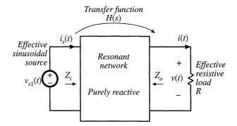
Fig. 19.30 Resonant inverter model.
