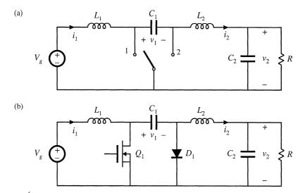
Fig. 2.20 Cuk converter: (a) with ideal switch, (b) practical realization using MOSFET and diode.
