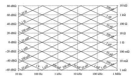
Fig. 8.49 "Reactance paper": an aid for graphical construction of impedances, with the magnitudes of various inductive, capacitive, and resistive impedances preplotted.
