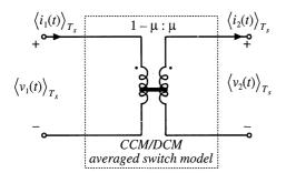
Fig. B.11 A general averaged switch model using the equivalent switch conversion ratio  $\mu$ .
