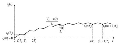
Fig. 2.11 Inductor current waveform during converter turn-on transient.
