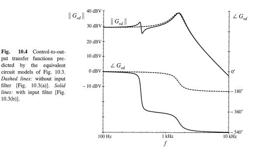
output transfer function  $G_{vd}(s)$ , the line-to-output transfer function  $G_{vg}(s)$ , and the converter output impedance  $Z_{out}(s)$ . Moreover, the influence of the input filter on these transfer functions can be quite severe.
