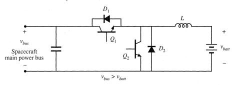
Fig. 4.15 Bidirectional battery charger/discharger, based on the dc-dc buck converter.
