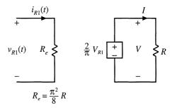
Fig. 19.21 An equivalent circuit for the rectifier and inductive filter network of the parallel resonant converter, which models the fundamental components of the rectifier ac input waveforms and the dc components of the load waveforms.
