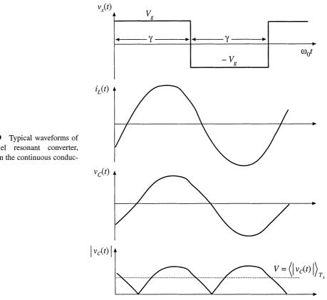
Fig. 19.49 Typical waveforms of the parallel resonant converter, operating in the continuous conduction mode.
