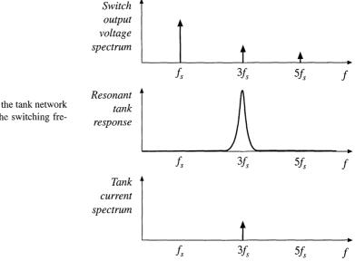
Fig. 19.17 Excitation of the tank network by the third harmonic of the switching frequency.
