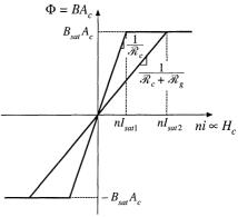
core, Fig. 13.12 has the same shape as the core B-H characteristic. When the core is not saturated,  $\Phi$  is related to *ni* according to the linear relationship of Eq. (13.28). When the core saturates,  $\Phi$  is equal to
