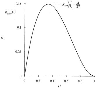
Fig. 5.13 Boost converter  $K_{crit}(D)$  vs. D.
