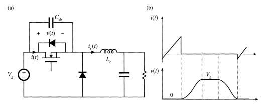
Fig. 20.7 Zero-voltage switching of a MOSFET, ZVS quasi-squarewave buck converter example. The MOSFET, its body diode, and its output capacitance  $C_{ds}$  are illustrated. (a) converter schematic, (b) MOSFET voltage and current waveforms.
