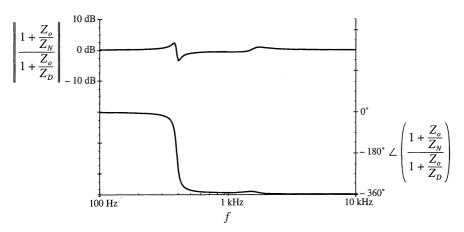
Fig. 10.14 Magnitude of the correction factor, Eq. (10.12), for the buck converter example of Fig. 10.8.
