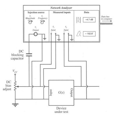
Fig. 8.59 Measurement of a transfer function.
