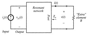
Fig. C.20 Application of the Extra Element Theorem to the system of Fig. C.19, to expose the dependence of  $Z_i(s)$  on R.
