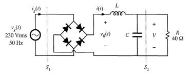
Fig. 16.13 Passive rectifier circuit of Problem 16.1
