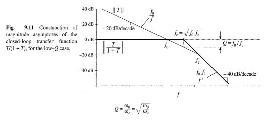
So the closed-loop response contains quadratic poles at  $f_c$ , the geometric mean of  $f_0$  and  $f_2$ . These poles have a low Q-factor when  $f_0 \ll f_2$ . In this case, we can use the low-Q approximation to estimate their frequencies:
