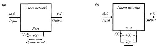
Fig. C.4 Modification of a linear network by addition of an extra element: (a) original system, (b) modified system, with impedance Z(s) connected at an electrical port.
