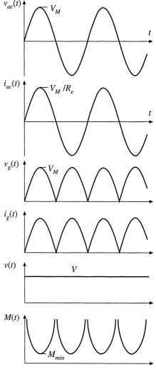
Fig. 18.4 Waveforms of the rectifier system of Fig. 18.3.
