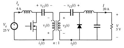
Fig. 15.5 Isolated Ćuk converter example.
