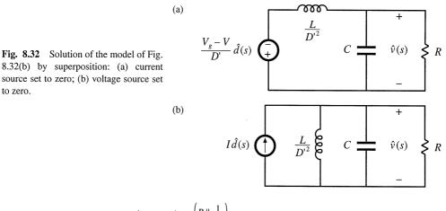
$$G_{vd}(s) = \left(-\frac{V_g - V}{D'}\right) \frac{\left(R \parallel \frac{1}{sC}\right)}{\frac{sL}{D'^2} + \left(R \parallel \frac{1}{sC}\right)} + I\left(\frac{sL}{D'^2} \parallel R \parallel \frac{1}{sC}\right)$$
