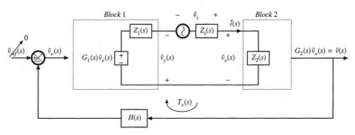
Fig. 9.35 Measurement of loop gain by voltage injection.
