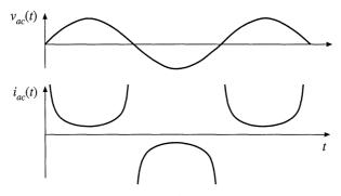
Fig. 18.28 Ac line current waveform of the single-phase ideal rectifier with output voltage feedback, when it supplies constant instantaneous power to a dc load. The THD tends to infinity, and the power factor tends to zero.
