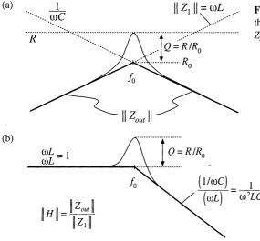
Fig. 8.51 Graphical construction of H and  $Z_{out}$  of the voltage divider circuit: (a) output impedance  $Z_{out}$ ; (b) transfer function H.
