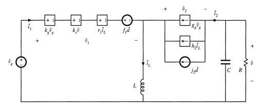
Fig. 11.22 A small-signal ac model of the DCM buck-boost converter.
