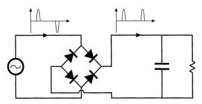
Fig. 16.6 Conventional peak detection rectifier.
