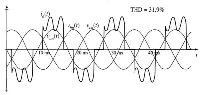
Fig. 17.9 Continuous conduction mode ac line-neutral voltages and phase *a* current, for a moderate value of inductance.
