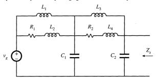
Fig. 8.69 Input filter circuit of Problem 8.13.
