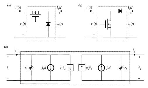
**Fig. 11.16** A convenient way to model the switch networks of DCM buck and boost converters: (a) defined terminal quantities of the DCM buck switch network, (b) defined terminal quantities of the boost switch network, (c) two-port small-signal ac model. The model parameters are given in Table 11.2.
