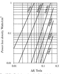
The parameters  $K_{fe}$  and  $\beta$  are determined by fitting Eq. (13.57) to the manufacturer's published data. Typical values of  $\beta$  for ferrite materials operating in their intended range of  $\Delta B$  and f lie
