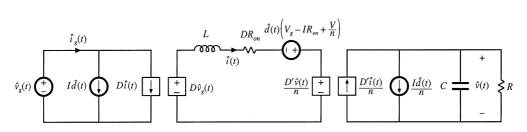
Fig. 7.26 The equivalent circuits of Figs. 7.23 to 7.25, collected together.
