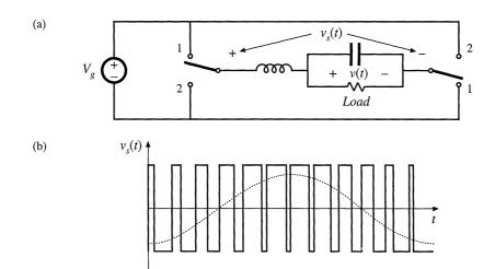
Fig. 1.13 A bridge-type dc-løac inverter: (a) ideal inverter circuit, (b) typical pulse-width-modulated switch voltage waveform  $v_s(t)$ , and its low-frequency component.
