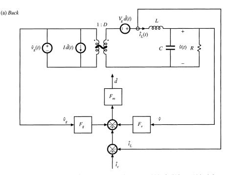
Fig. 12.25 More accurate models of current-programmed converters: (a) buck, (b) boost, (c) buck-boost.
