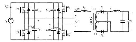
Fig. 20.36 Zero-voltage transition converter, based on the full-bridge isolated buck converter.
