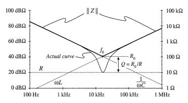
Fig. 8.44 Actual impedance magnitude (solid line) for the series resonant R-L-C example. The inductor and capacitor impedances cancel out at  $f = f_0$ , and hence  $Z(j\omega_0) = R$ .
