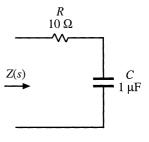
**Fig. 8.38** Series *R*–*C* network example.
