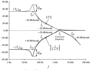
**Fig. 9.7** Graphical construction of || 1/(1 + T) ||. quencies is
