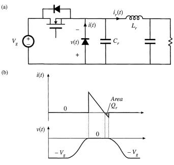
**Fig. 20.4** Zero-voltage switching at the turn-off transition of a diode, ZVS quasi-squarewave buck converter example: (a) converter schematic, (b) diode current and voltage waveforms.
