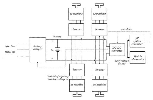
Fig. 1.16 An electric vehicle power and drive system.
