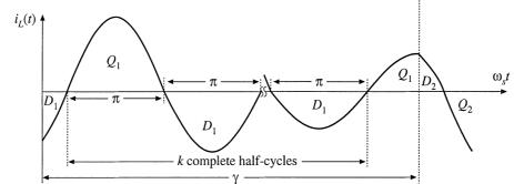
Fig. 19.41 Continuous conduction modes of the series resonant converter: (a) switching frequency ranges over which various mode indices k and subharmonic numbers  $\xi$  occur; (b) tank inductor current waveform, type k CCM, for odd k; (c) tank inductor current waveform, type k CCM, for even k.
