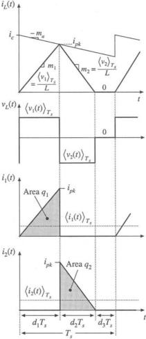
**Fig. 12.31** Waveforms, CPM DCM buck–boost example.
