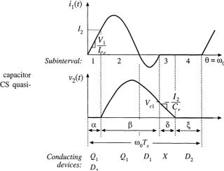
Fig. 20.18 Tank inductor current and capacitor voltage waveforms, for the full-wave ZCS quasi-resonant switch cell of Fig. 20.8(d).
