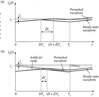
Fig. 12.11 When noise perturbs a controller signal such as  $i_c$ , a perturbation in the duty cycle results: (a) with no artificial ramp and small inductor current ripple, the perturbation  $\hat{d}$  is large; (b) an artificial ramp reduces the controller gain, thereby reducing the perturbation  $\hat{d}$ .
