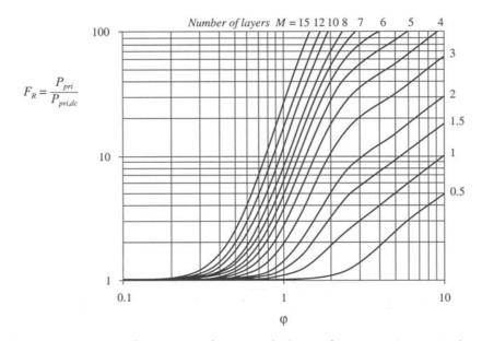
Fig. 13.34 Increased total winding copper loss in the two-winding transformer example, as a function of  $\varphi$  and number of layers *M*, for sinusoidal excitation.
