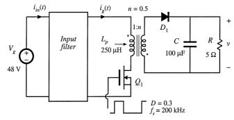
Fig. 10.30 Flyback converter, Problems 10.1, 10.4, 10.6, 10.8, and 10.10.
