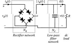
ple approximation as usual:  $v(t) \approx V$ ,  $i(t) \approx I$ . The diode rectifiers switch when  $i_R(t)$  passes through zero, as shown in Fig. 19.11. The rectifier input voltage  $v_R(t)$  is essentially a square wave, equal to + v(t) when  $i_R(t)$  is positive and - v(t) when  $i_R(t)$  is negative. Note that  $v_R(t)$  is in phase with  $i_R(t)$ .
