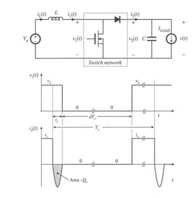
Fig. 7.72 Boost converter and waveforms illustrating reverse recovery of the diode. Averaged switch modeling in this converter is addressed in Problem 7.19.
