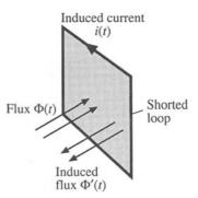
**Fig. 13.3** Illustration of Lenz's law in a shorted loop of wire. The flux  $\Phi(t)$  induces current i(t), which in turn generates flux  $\Phi'(t)$  that tends to oppose changes in  $\Phi(t)$ .
