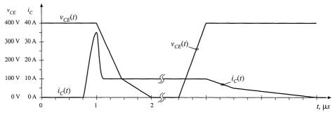
Fig. 4.57 IGBT voltage and current waveforms, Problem 4.7.
