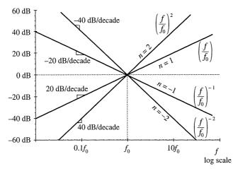
Fig. 8.3 Magnitude Bode plots of functions which vary as  $f^n$  are linear, with slope *n* dB per decade.
