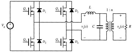
Fig. C.13 Parallel resonant inverter example.
