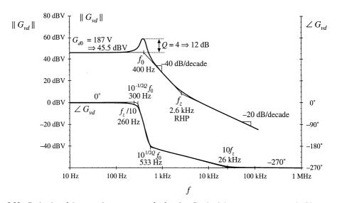
Fig. 8.33 Bode plot of the control-to-output transfer function  $G_{vd}$ , buck-boost converter example. Phase reversal owing to output voltage inversion is not included.
