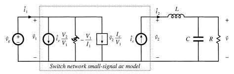
Fig. 12.19 Small-signal model of the CCM CPM buck converter, derived by perturbation and linearization of the switch network in Fig. 12.17.
