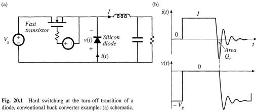
(b) diode voltage and current waveforms.
