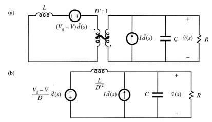
Fig. 8.31 Manipulation of buck-boost equivalent circuit to find the control-to-output transfer function  $G_{vd}(s)$ : (a) set  $\hat{v}_e$  source to zero; (b) push inductor and voltage source through transformer.
