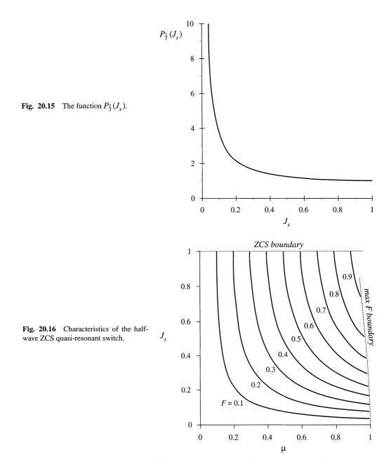
of the current  $I_2$ , via  $J_s$ . The characteristics end at  $J_s = 1$ ; according to Eq. (20.31), the zero current switching property is lost when  $J_s > 1$ . The characteristics also end at the maximum switching frequency limit given by Eq. (20.31). This expression can be simplified by use of Eq. (20.43), to express the limit in terms of  $\mu$  as follows:
