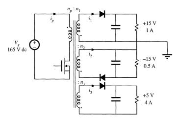
Fig. 6.46 Three-output flyback converter design, Problem 6.10.
