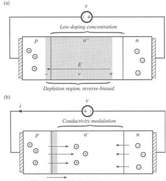
**Fig. 4.24** Power diode: (a) under reverse-bias conditions, (b) under forward-bias conditions.
