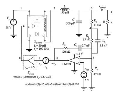
Fig. B.15 Buck voltage regulator example.
