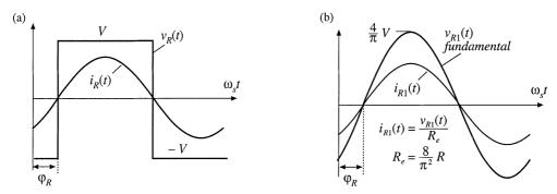
Fig. 19.11 Rectifier network input terminal waveforms: (a) actual waveforms  $v_R(t)$  and  $i_R(t)$ , (b) fundamental components  $v_{R1}(t)$  and  $i_{R1}(t)$ .
