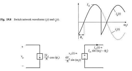
Fig. 19.9 An equivalent circuit for the switch network, which models the fundamental component of the output voltage waveform and the dc component of the input current waveform.
