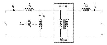
Fig. 13.18 Two-winding transformer equivalent circuit, including magnetizing inductance referred to primary, and primary and secondary leakage inductances.
