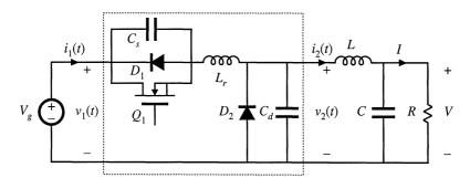
Fig. 20.26 Half-wave ZVS multiresonant buck converter.
