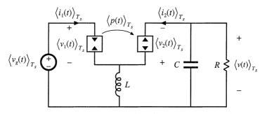
Fig. 12.32 CPM DCM buck-boost converter model, derived via averaged switch modeling.
