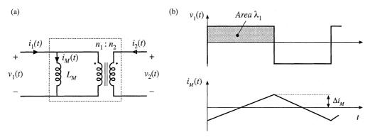
Fig. 13.45 Conventional transformer: (a) equivalent circuit, (b) typical primary voltage and magnetizing current waveforms.
