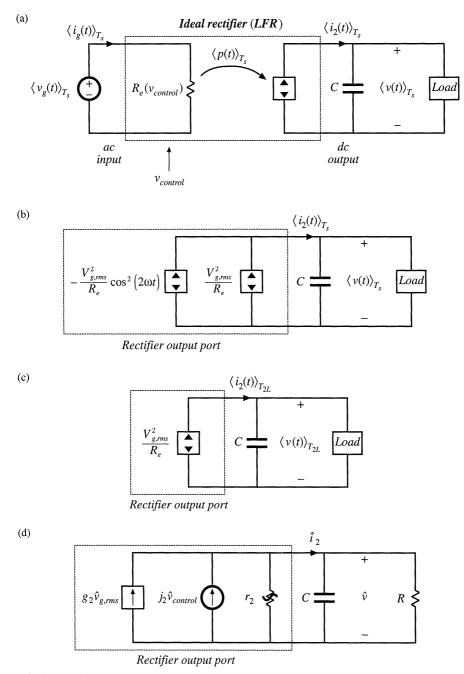
**Fig. 18.29** Steps in the derivation of low-frequency small-signal rectifier model: (a) large-signal LFR model, averaged over one switching period  $T_s$ ; (b) separation of power source into its constant and time-varying components; (c) removal of second-harmonic components by averaging over one-half of the ac line period,  $T_{2L}$ ; (d) small-signal model obtained by perturbation and linearization of Fig. 18.29(c).
