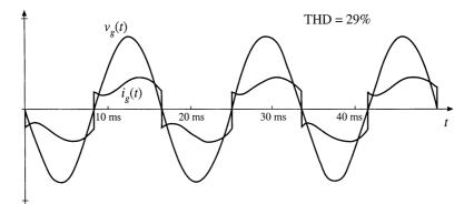
Fig. 17.2 Typical ac line current and voltage waveforms, continuous conduction mode.  $f_0/f_L = 5$ , Q = 0.25.
