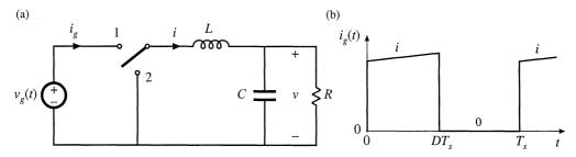
Fig. 10.1 Buck converter example: (a) circuit of power stage, (b) pulsating input current waveform.
