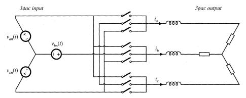
Fig. 4.21 A 3øac-3øac matrix converter, which requires nine SPST four-quadrant switches.
