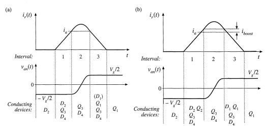
Fig. 20.42 Waveforms of the ARCP circuit of Fig. 20.41: (a) basic waveforms, (b) with current boost.
