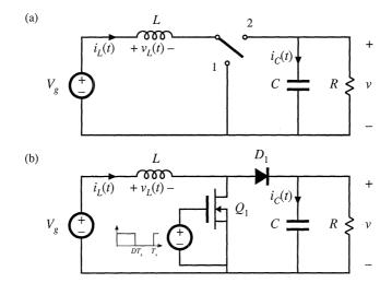
Fig. 2.13 Boost converter: (a) with ideal switch, (b) practical realization using MOSFET and diode.
