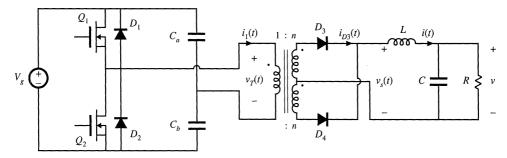
Fig. 6.20 Half-bridge transformer-isolated buck converter.
