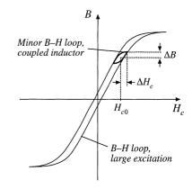
Fig. 13.48 Coupled inductor minor *B*-*H* loop.
