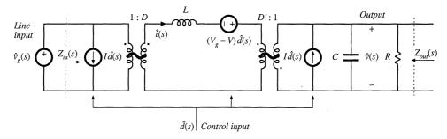
Fig. 8.1 Small-signal equivalent circuit model of the buck-boost converter, as derived in Chapter 7.
