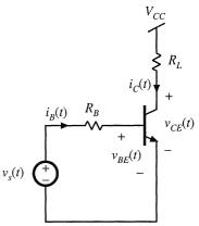
**Fig. 4.31** Circuit for BJT switching time example.
