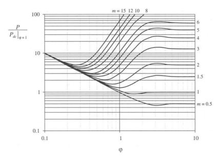
Fig. 13.32 Layer copper loss, relative to the dc loss in a layer having effective thickness of one penetration depth.
