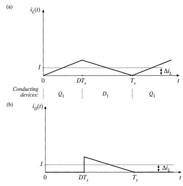
Fig. 5.3 Buck converter waveforms at the boundary between the continuous and discontinuous conduction modes: (a) inductor current  $i_{I}(t)$ , (b) diode current  $i_{D}(t)$ .
