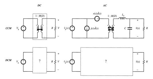
Fig. 11.1 The objective of this chapter is the derivation of large-signal dc and small-signal ac equivalent circuit models for converters operating in the discontinuous conduction mode.
