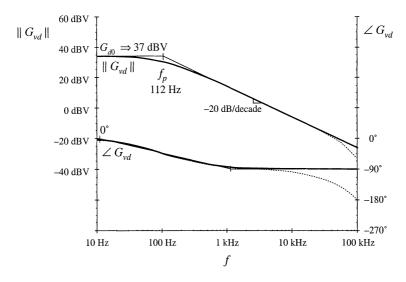
Fig. 11.19 Magnitude and phase of the control-to-output transfer function, DCM boost example. Solid lines: function and its asymptotes, approximate single-pole response predicted by the model of Fig. 11.18. Dashed lines: more accurate response that includes high-frequency inductor dynamics.
