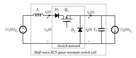
Fig. 20.9 The half-wave ZCS quasi-resonant switch cell, driven by the terminal quantities  $\langle v_1(t) \rangle_{T_s}$  and  $\langle i_2(t) \rangle_{T_s}$ .
