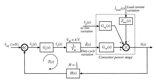
Fig. 9.25 System block diagram, design example.
