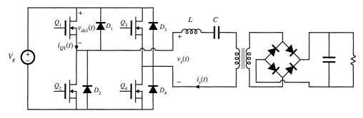
Fig. 19.24 A series resonant converter incorporating a full-bridge switch network.
