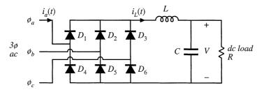
Fig. 17.7 Basic uncontrolled 3ø bridge rectifier circuit, with dc-side L-C filter.
