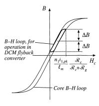
Fig. 13.50 Operational *B*–*H* loop of a DCM flyback transformer.
