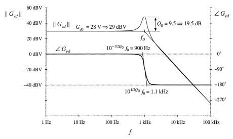
Fig. 9.24 Converter small-signal control-to-output transfer function  $G_{vd}$ , design example.
