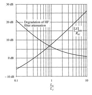
**Fig. 10.23** Performance attained via optimal design procedure, parallel  $R_{f}$ - $L_{b}$  circuit of 10.20(b). Optimum peak filter output impedance  $||Z_{o}||_{mm}$  and increase of filter high-frequency gain, vs.  $n = L_{b}/L$ .
