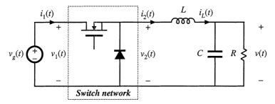
Fig. 12.16 Averaged switch modeling of a current-programmed converter: CCM buck example.
