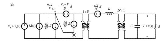
Fig. 7.60 Steps in the manipulation of the buck-boost ac model into canonical form.
