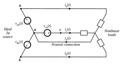
Fig. 16.9 Current flow in a three-phase four-wire network.
