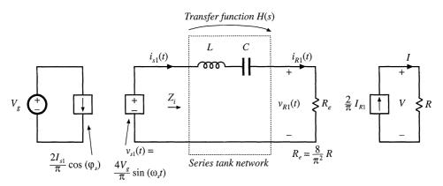
Fig. 19.15 Steady-state equivalent circuit of the series resonant converter.
