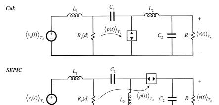
Fig. 11.11 Averaged large-signal equivalent circuits of five basic converters operating in the discontinuous conduction mode.
