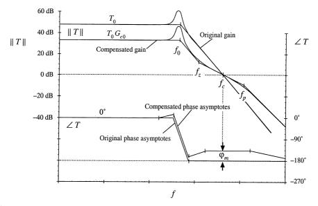
Fig. 9.17 Compensation of a loop gain containing two poles, using a lead (*PD*) compensator. The phase margin  $\varphi_m$  is improved.
