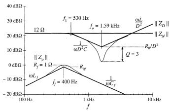
Fig. 10.18 Impedance design criteria  $||Z_N(j\omega)||$  and  $||Z_D(j\omega)||$  from Fig. 10.10, with the filter output impedance  $||Z_a(j\omega)||$  of Fig. 10.17(b) superimposed. The design criteria of Eq. (10.13) are well satisfied.
