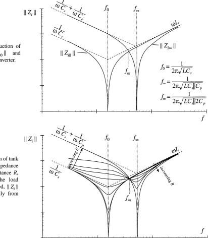
**Fig. 19.35** Construction of the quantities  $||Z_{i0}||$  and  $||Z_{i\infty}||$ , for the LCC inverter.
