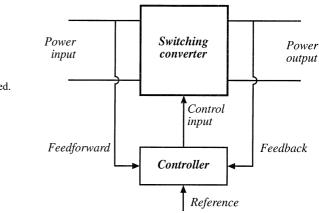
Fig. 1.2 A controller is generally required.
