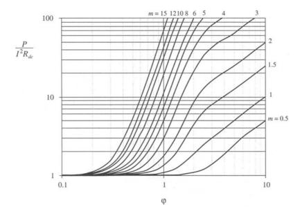
Fig. 13.31 Increase of layer copper loss due to the proximity effect, as a function of  $\varphi$  and MMF ratio *m*, for sinusoidal excitation.
