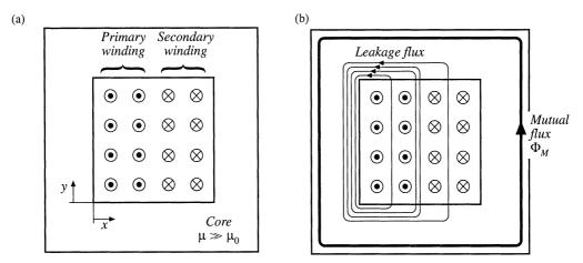
Fig. 13.26 Two-winding transformer example: (a) core and winding geometry, (b) typical flux distribution.
