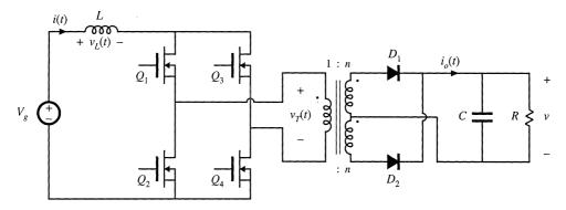
Fig. 6.34 Full-bridge transformer-isolated boost converter.
