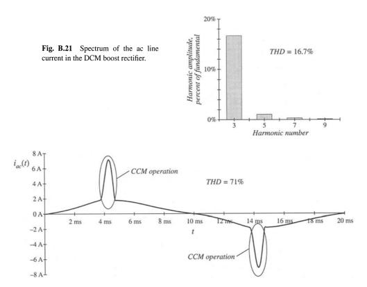
Fig. B.22 Ac line current of the DCM boost rectifier example, when the output is overloaded.
