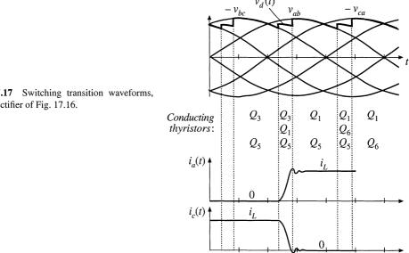
Fig. 17.17 Switching transition waveforms, for the rectifier of Fig. 17.16.
