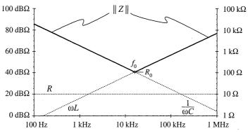
Fig. 8.43 Graphical construction of impedance asymptotes for the series R-L-C network example, with R decreased to  $10 \Omega$ .
