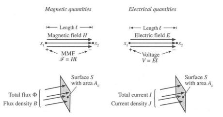
Fig. 13.1 Comparison of magnetic field H, MMF  $\Phi$ , flux  $\mathscr{F}$ , and flux density B, with the analogous electrical quantities E, V, I, and J.
