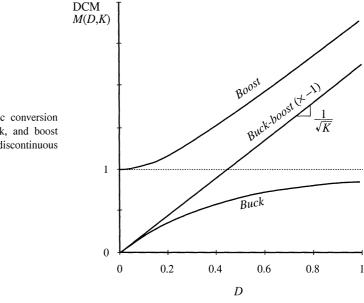
Fig. 5.20 Comparison of dc conversion ratios of the buck–boost, buck, and boost converters operated in the discontinuous conduction mode.
