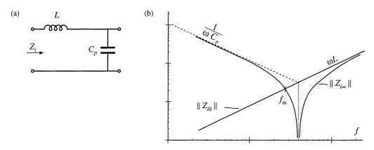
Fig. 19.33 Tank network, parallel resonant converter example: (a) tank circuit, (b) Bode plot of input impedance magnitude  $||Z_i||$  for the limiting cases  $R \to 0$  and  $R \to \infty$ .
