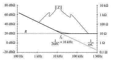
Fig. 8.40 Construction of the composite asymptotes of ||Z||. The asymptotes of the series combination can be approximated by simply selecting the larger of the individual resistor and capacitor asymptotes.
