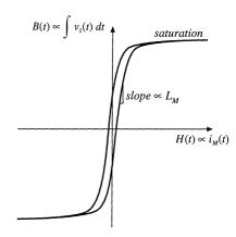
Fig. 6.17 *B*-*H* characteristics of transformer core.
