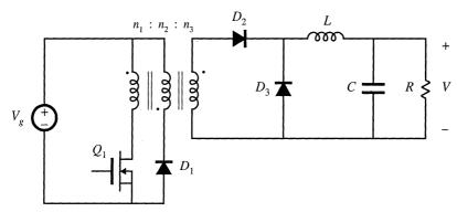
Fig. 6.22 Single-transistor forward converter.
