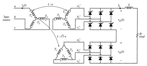
Fig. 17.31 Twelve-pulse rectifier circuit, with one controlled and one uncontrolled bridge, Problem 17.7.
