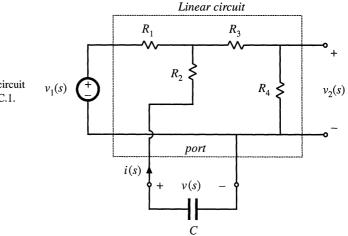
**Fig. C.11** Manipulation of the circuit of Fig. C.10 into the form of Fig. C.1.
