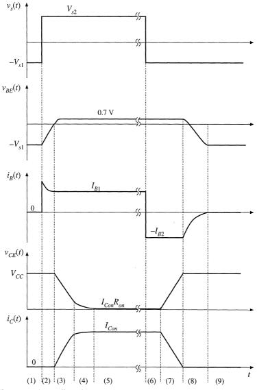
Fig. 4.32 BJT turn-on and turn-off transition waveforms.
