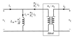
Fig. 13.16 Transformer model including magnetizing inductance.
