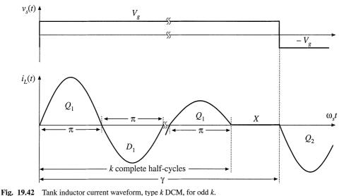
normally purposely designed to operate in odd discontinuous conduction modes, because the output voltage is not controllable. Nonetheless, when the load is removed with  $f_s < f_0$ , the series resonant converter operates in k = 1 DCM with M = 1.
