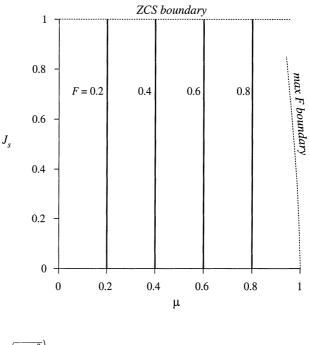
**Fig. 20.19** Characteristics of the full-wave ZCS quasi-resonant switch.
