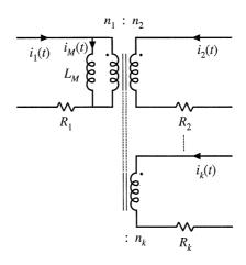
Fig. 15.4 Computed elements of simple transformer model.
