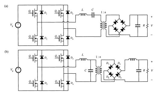
Fig. 19.40 Transformer-isolated resonant dc-dc converters: (a) series resonant converter, (b) parallel resonant converter.
