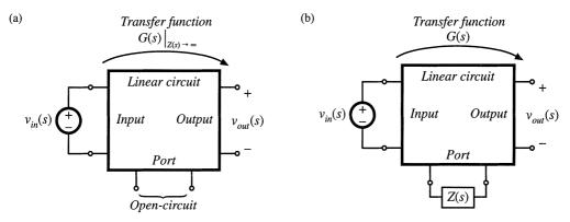
Fig. C.1 How an added element changes a transfer function G(s): (a) original conditions, before addition of the new element; (b) addition of element having impedance Z(s).
