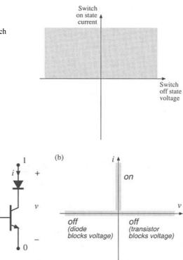
Fig. 4.16 Voltage-bidirectional two-quadrant switch properties.
