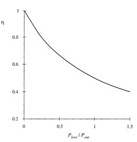
Fig. 1.3 Converter power loss vs. efficiency.
