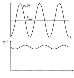
as an electrolytic capacitor. The difference between the instantaneous input and load powers flows through this capacitor.
