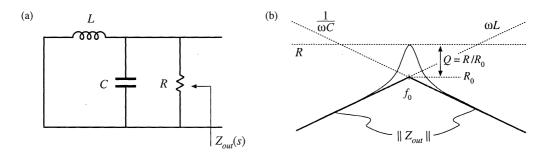
Fig. 8.54 Construction of buck converter output impedance  $Z_{out}(s)$ : (a) circuit model; (b) impedance asymptotes.
