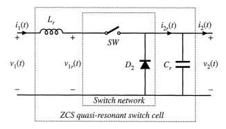
Fig. 20.20 Basic ZCS quasi-resonant switch cell.
